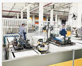
Robotic Welding for Inner and Outer Tubes 内外管机器人焊接焊接
